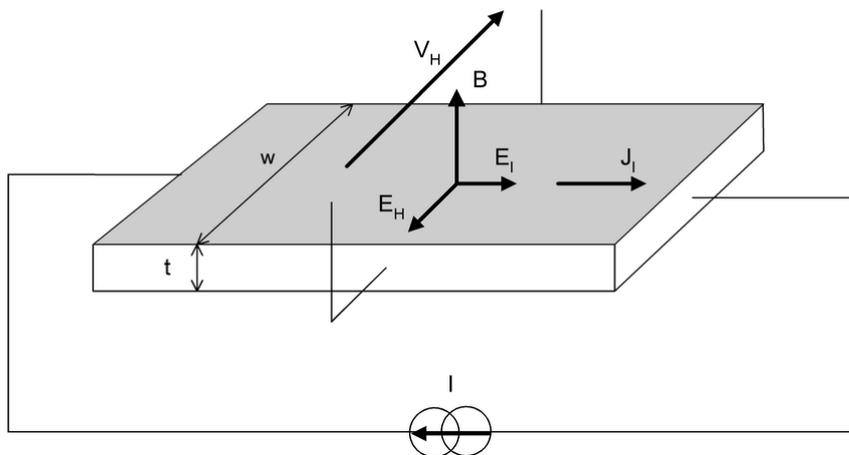
Principle: a conductor plate is fed with an electrical current. When this plate is located close to magnetic field (B) that is perpendicular to the plate (B is vertical here), the Hall effect generates a voltage  $V_H$  that is proportional to the intensity of the magnetic field.
