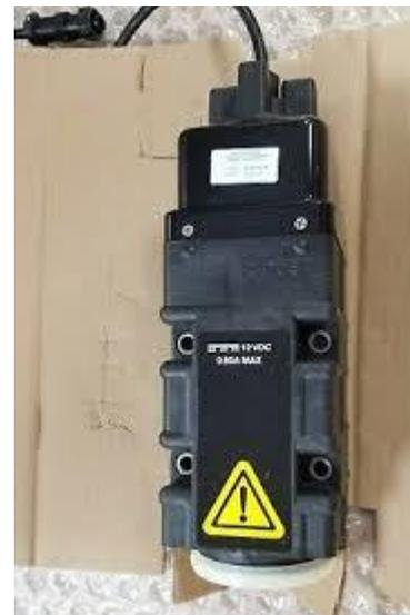
The Radar generates a signal at a frequency of 2.4 GHz that corresponds to microwave wavebands. The signal is reflected by the ground and part of it is travelling back to the sensor. When the tractor is immobile, it acts like a telemeter. When the tractor moves, the delay between the emission and the reception is proportional to the travel speed.
