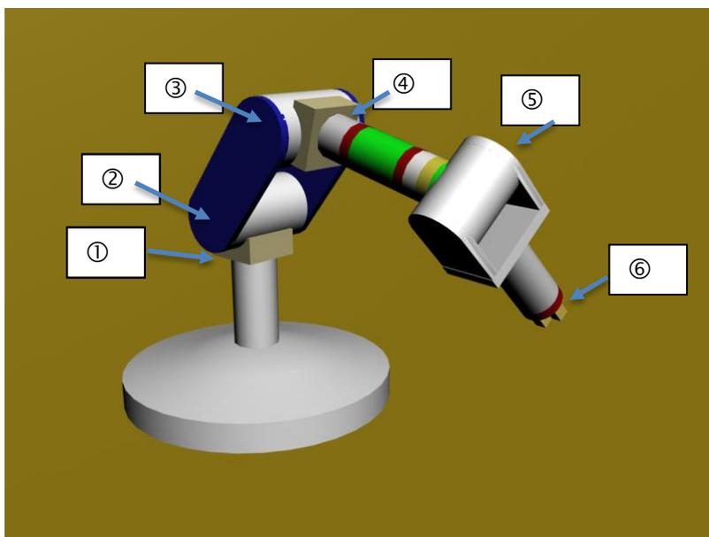
As only 1 axis (X,Y or Z) is allowed for each pivot only one degree of freedom is provided by each pivot.
